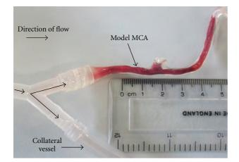
FIGURE 3: MCA with thrombus loaded and collateral vessel displayed.
