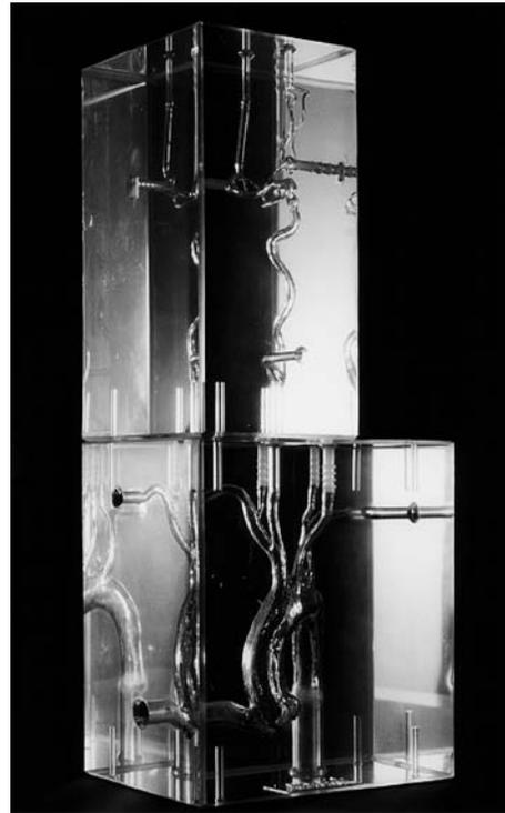
**Fig. 1** Photograph of the right carotid artery rigid model with three aneurysms located at the origin of the posterior communicating artery, in the anterior communicating artery, and at the bifurcation of the middle cerebral artery. The silicone block can be connected to an aortic arch silicone block with a simple "push and pull" connection system. The white obturators are connected to each aneurysm cavity.
